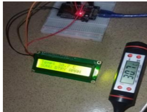
Gambar 5. Kalibrasi sensor suhu
